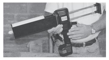
5.4 Push rack forward until pistons make contact with back of cartridge, close clutch. NOTE: Remember to condition the material to at least 65° F (18°C) prior to using!
